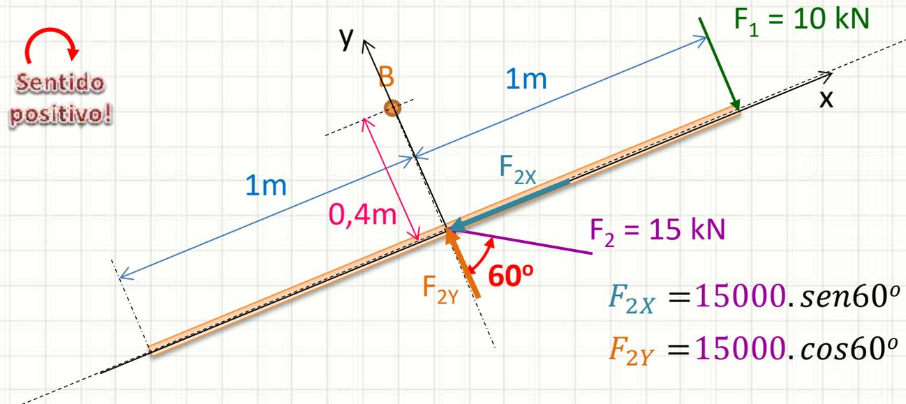
$$F_{2X} = 15000 \cdot \text{sen}60^\circ = 13 \text{ kN.m}$$
