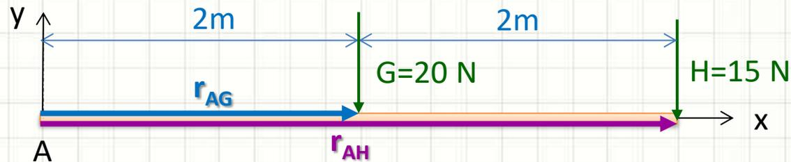
$$\vec{M}_{AG} = \det \begin{vmatrix} \vec{i} & \vec{j} & \vec{k} \\ r_x & r_y & r_z \\ F_x & F_y & F_z \end{vmatrix} = \begin{vmatrix} \vec{i} & \vec{j} & \vec{k} \\ 2 & 0 & 0 \\ 0 & -20 & 0 \end{vmatrix} = -40\vec{k}$$
