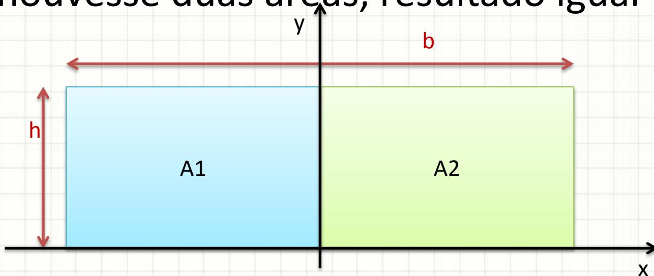
$$\begin{aligned}I_x &= \int_{A1} y^2 \cdot dA + \int_{A2} y^2 \cdot dA = \int_0^h y^2 \cdot \frac{b}{2} \cdot dy + \int_0^h y^2 \cdot \frac{b}{2} \cdot dy = \\&= \frac{b \cdot h^3}{6} + \frac{b \cdot h^3}{6} = \frac{b \cdot h^3}{3}\end{aligned}$$
