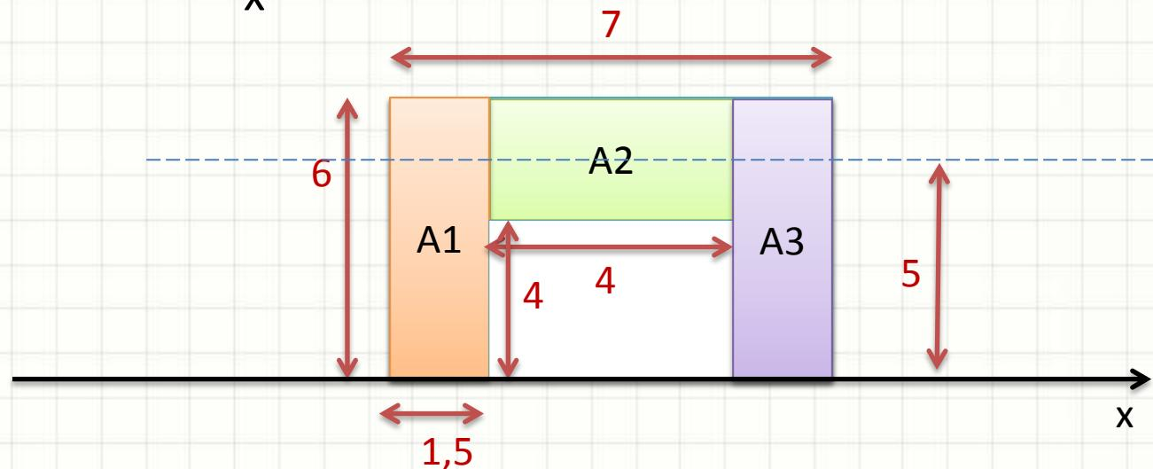
$$I_x = I_{A1x} + I_{A2x} + I_{A3x}$$
