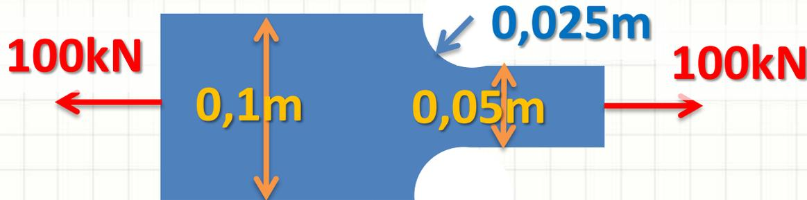
$$\begin{aligned} A &= 0,01 \text{ m}^2 \\ A_R &= 0,005 \text{ m}^2 \\ \sigma_{\text{lim}} &= 24 \text{ MPa} \end{aligned}$$
