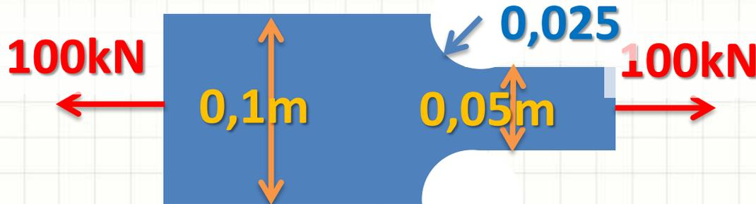
$$\begin{aligned} A &= 0,01 \text{ m}^2 \\ A_R &= 0,005 \text{ m}^2 \\ \sigma_{lim} &= 24 \text{ MPa} \end{aligned}$$
